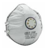
Face mask with activated carbon and exhalation valve, to protect the airways against dust, mist and fumes with TLV>0.1 mg/m3. Vapors, gases and unpleasant odors are captured by the activated carbon filter. Protection class: FF P2 (EN 149:2001). Usage limit for dust 10XTLV, for gas and vapors <TLV. CE certified.
