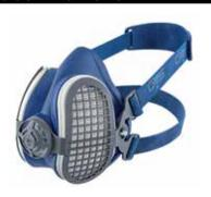
Mask body made in TPE thermoplastic elastomer (Elipse edition). It adapts and adheres perfectly to the user's face, preventing dust from infiltrating the interstices created by poor adherence between the user's face and the mask. The large front non-return valve allows to minimize the user's breathing resistance and moisture build-up inside the mask.
