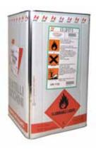
Super spray monocomponent neoprene adhesive. Suitable for gluing foam pads together, wood, metals and plastics. Apply on both parts using spray equipment and press them together.
