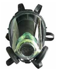
Full-face mask made from FDA approved (BLS 5500) TPE. Polycarbonate visor, optical class 1 tested (EN 166). Anti-scratch treatment. Exhalation valve with anti-splash cover.
