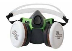
Oronasal half-mask respirator made from thermoplastic rubber, with 019SA2R01 and 019SP2R01 filters for protection against gases, organic vapors and dust. Protection class: A2 (EN 14387:2004). CE certified.
