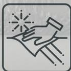
The surfaces coated with **AOX** and **OPX** series products are able to self-heal by gently wiping them with a damp or wet cloth using warm water. The **OPX** film can also be repaired by heating the damaged surface with a hair dryer for 30" and then rubbing with a wet cloth.
